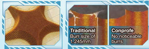
Material: Nomex Honeycomb Feature: Contouring
