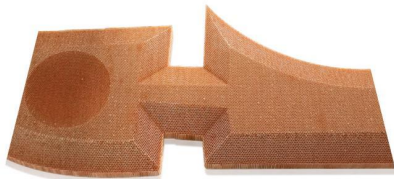
Nomex honeycomb Small angle (<20 °) contour machining
