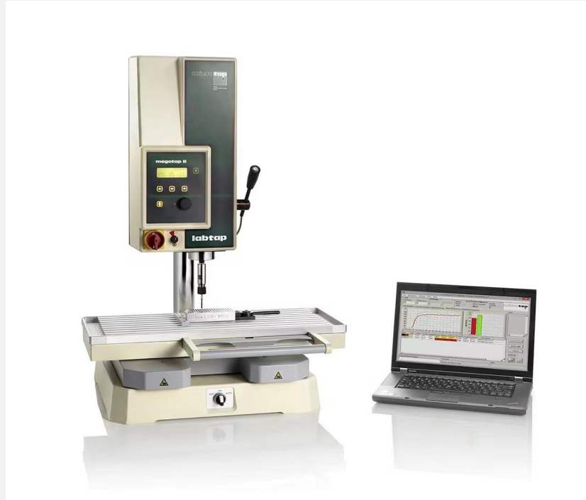
Test of MQL oil's lubricity
